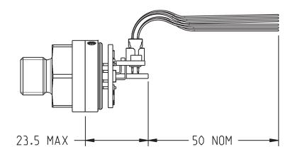
GAUGE SENSOR WITH PB PRESSURE CONNECTOR SHOWN
